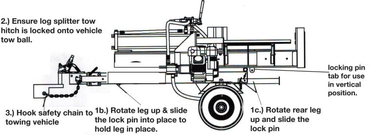
Remember to turn the engine fuel tap off prior to towing to prevent flooding of the engine.
