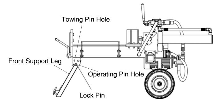
Remove the Lock Pin (14) from the Towing Pin Hole (16) and lower the Front Support Leg (10). While making sure that the Front Support Leg (10) is on the floor, connect the Lock Pin (14) to the Operating Pin Hole (15) and secure tightly.
