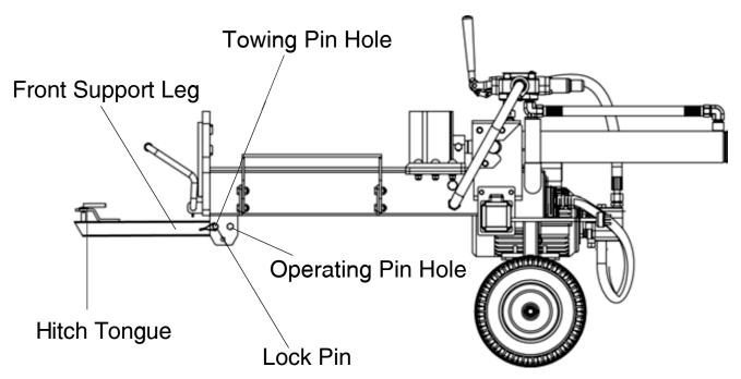
While towing, raise the Front Support Leg (10) and connect the Hitch Tongue (13) to your vehicle. The Lock Pin (14) should then be removed from the Operating Pin Hole (15) and inserted in the Towing Pin Hole (16).
