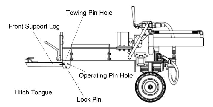
While towing, raise the Front Support Leg (10) and connect the Hitch Tongue (13) to your vehicle. The Lock Pin (14) should then be removed from the Operating Pin Hole (15) and inserted in the Towing Pin Hole (16).
