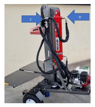
Secure Hose C on valve block to Hose D on the cylinder.
