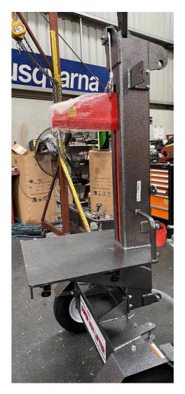
Note: Ensure assembly is stable by keeping the lifting equipment attached until the Y frame is attached.
