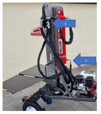
Secure Hose E on valve block to Hose F on the cylinder.
