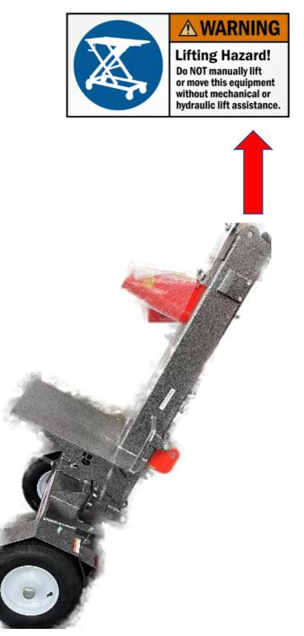
Lift from eyelet in main frame using a suitable gantry or similar.
