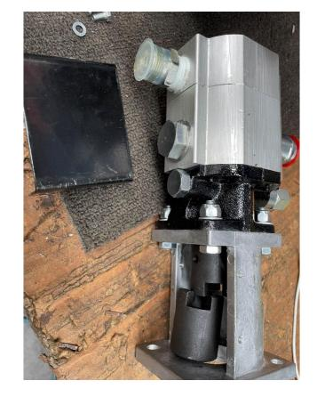
Fitting the pump to the engine - Take small black guard off the pump spider gear casing.
