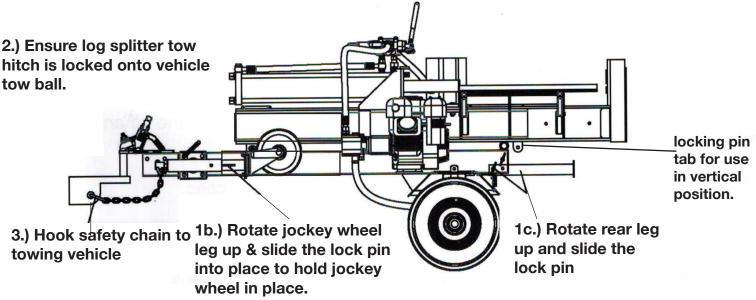
Remember to turn the engine fuel tap off prior to towing to prevent flooding of the engine.
