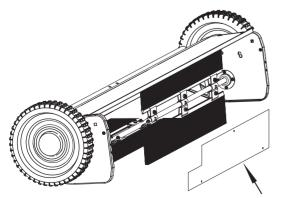
Four wood splints are used to protect the brushes during shipping.
